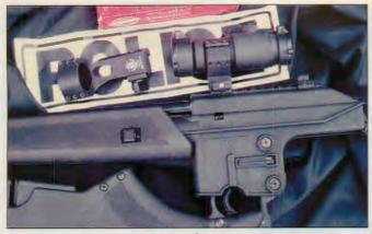
The Aimpoint Comp ML2 Sight was mounted on the SU-16 using the new mount from World Wide Ordnance. WWO's extended-eyerelief mount is also shown. (below) As a compact weapon, the SU-16D compares favorably with an M4 in the collapsed mode.
